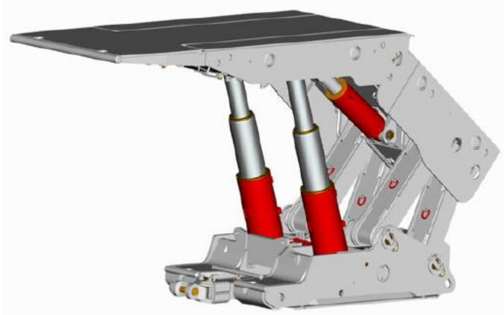
Figure 23. Model view of powered roof support
