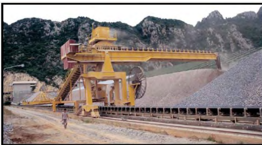
Figure 2-33: Stacking at coal stocking yards using stacker-reclaimer (typical)
